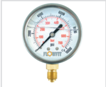
Dual scale psi (outer) in black and bar (inner) in red
